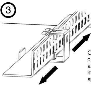
Once properly installed, clips will slide freely along rail to allow maximization of shelf space.
