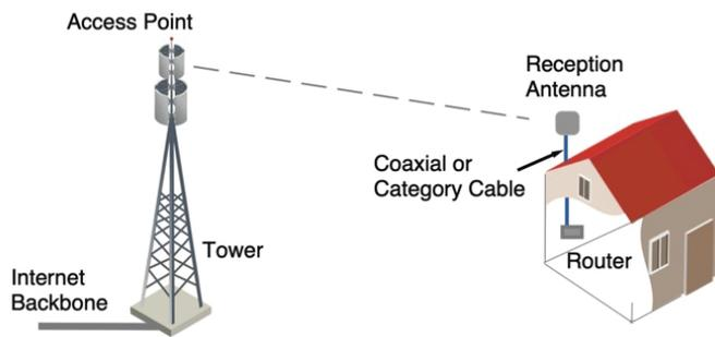
At the subscriber's location, a reception antenna brings the broadband signal into the premises over coaxial or category cable connected to a router. The trend for customer premises deployments is the use of self-installation kits. Category cables (Cat5e, Cat6, etc.) are the most common method of connecting the reception antenna to a router. A quick entry into the premises can be made using a clever flat window/door jumper from Amphenol Broadband
