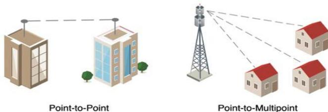
A point-to-point connects two locations such as a tower network on the internet backbone and a business or residential building. While point-to-multipoint FW networks use a single donor antenna to connect to multiple locations, each with its own reception dish. Campus environments are a great example of an area that may be effectively served using multi-point FW.
